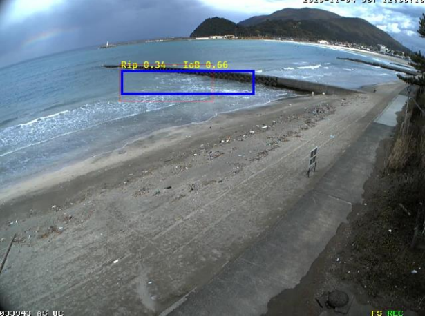
Fig.17 Examples of rip current detection by AI Model A-2 compared with the annotation area for Cam 03.
