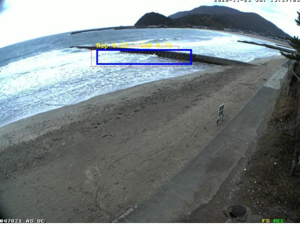
Fig.17 Examples of rip current detection by AI Model A-2 compared with the annotation area for Cam 03.
